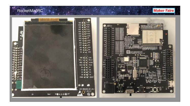
This is Espressiv's ESP-WROVER-KIT with FTDI debugger on board.
