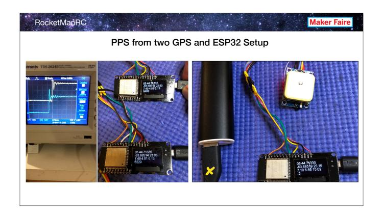
The PPS from two GPS stay within 50 ns of each other even during very degraded satellite reception.
