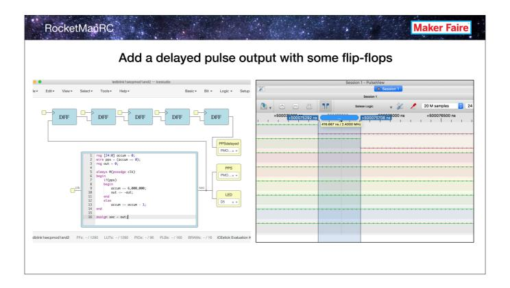
This simulates the ESP32 interrupt response so we know we have our setup correct.
