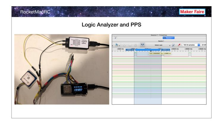
Why it is not exactly 1 second is due to the clock in the logic analyzer. But it's good enough for this.
