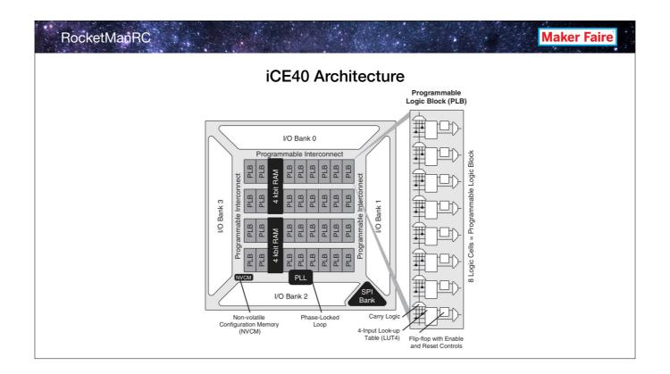
Essentially an array of programmable logic blocks that are configured by "programming".
